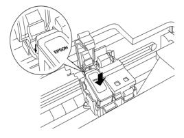
8. Push the clamp down until it locks firmly into place.
